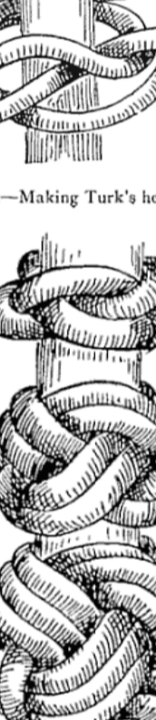
FIG. 120.—French shroud knot (complete).
