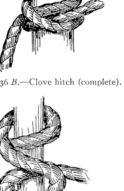
FIG. 33.—Slippery hitch (tying).
