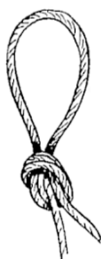
FIG. 62.—Loop knot. FIG. 63.—Loop knot. FIG. 64.—Loop knot.
